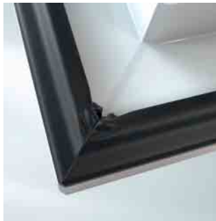
Conventional sealing technology forms hard corners when welded. This results in a loss of elasticity and hence reduced weathertightness.
