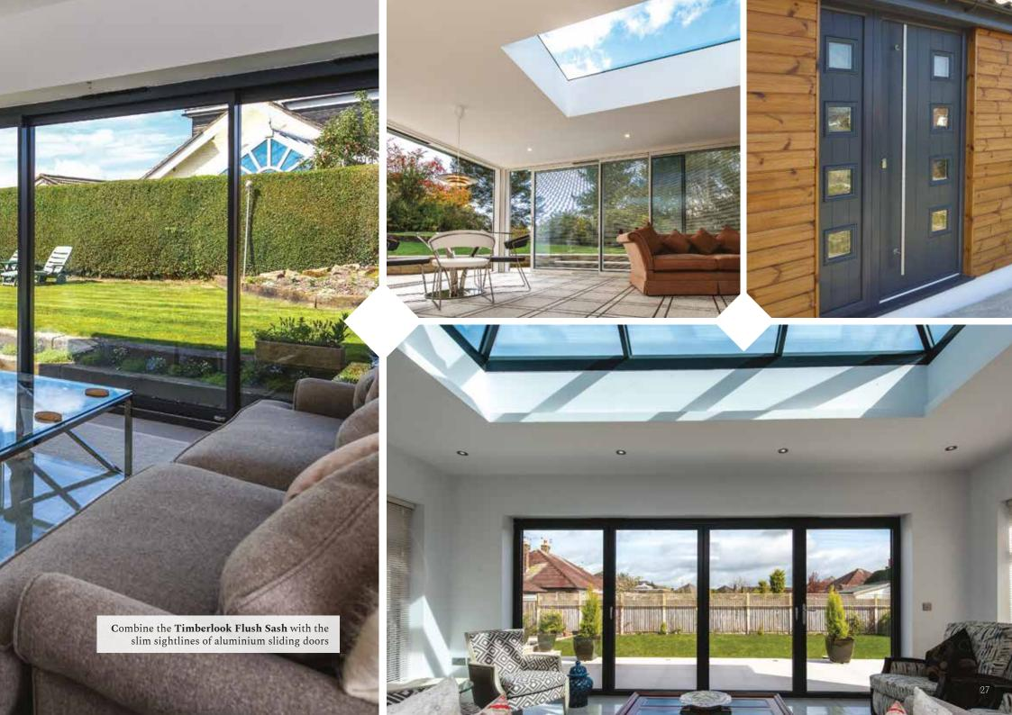
Timberlook is a uPVC window system that successfully replicates traditional wooden windows, with the authentic appearance of a mortise and tenon joint. It is ideal for period, character, or historic projects, and has be accepted as a timber alternative for renovations and new-build developments in conservation areas by local planning authorities.
