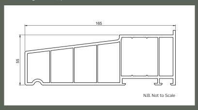
Old imperial bricks varied in height, while modern metric bricks measure 65mm, and old timber cills were deep and often aligned with a course of bricks. The Radlington Cill, at 55mm, is a modern interpretation that allows for packing expansion, bay pole jacks, and irregular mortar.
